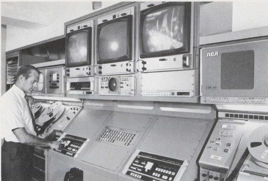
The latest advance in electronic editing of video tape is represented in these new time-code editing systems, from RCA. Each editing panel, the one on the left shown being operated, controls one tape machine.
